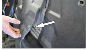
3. Pull back the inner lower corners of the back panels to gain access and remove the two air filter housing mounting bolts.
