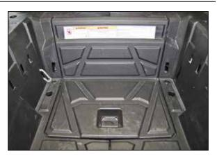
4. Release and lift off the engine cover.
