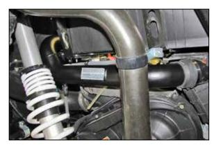
22. Feed the intake tube assembly behind the clutch intake hose and then install it into the intake plenum coupler and then into the filter coupler. Adjust the tube for best fit and then secure with the provided hose clamps.
