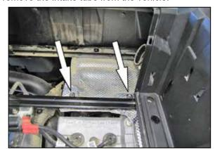
9. Remove the two nuts and bolts shown that secure the heat shielding to the chassis.
