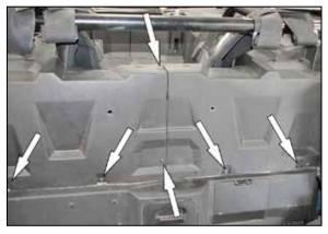
12. Reinstall six of the eight bolts removed in step #2. Reinstall the seats.
